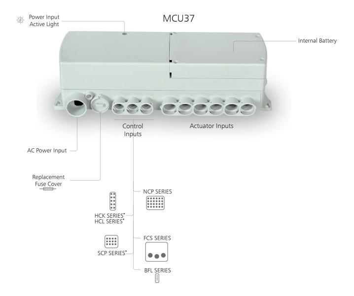
HCK SERIES\*, HCL SERIES\* and SCP SERIES\* are only usable with 180 degree cable. Please review the HCK, HCL and SCP datasheet for detailed information.
